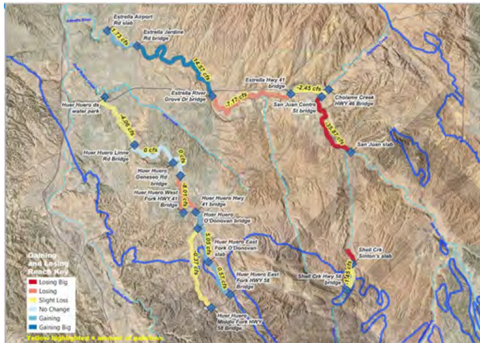
Figure 7. Synoptic streamflow measurements gain / loss estimates (GSI Water Solutions, 2023)
